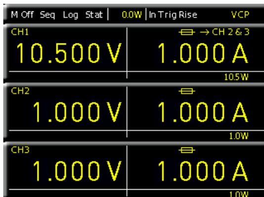
Fig. 5.4: Fuse Linking example
