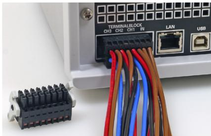
Fig. 6.2: Example plug-in terminal block connector
