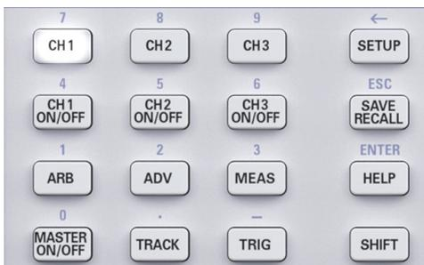
Fig. 4.2: Numeric keypad with function keys
