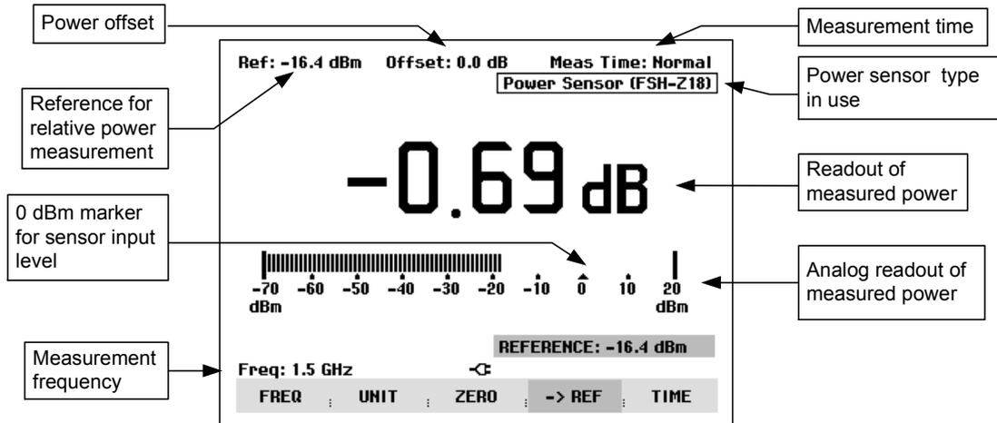
The power sensor has a memory containing frequency-dependent correction values. This means that the highest accuracy is reached for signals whose frequency is known. If the R&S FSH switches over to the power measurement mode from another operating mode, it uses the center frequency as the frequency for the power sensor.
