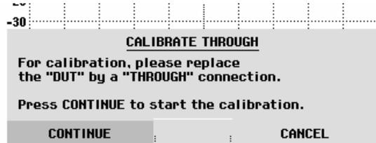
During calibration, the R&S FSH outputs the message "Calibrating THROUGH, please wait...".
