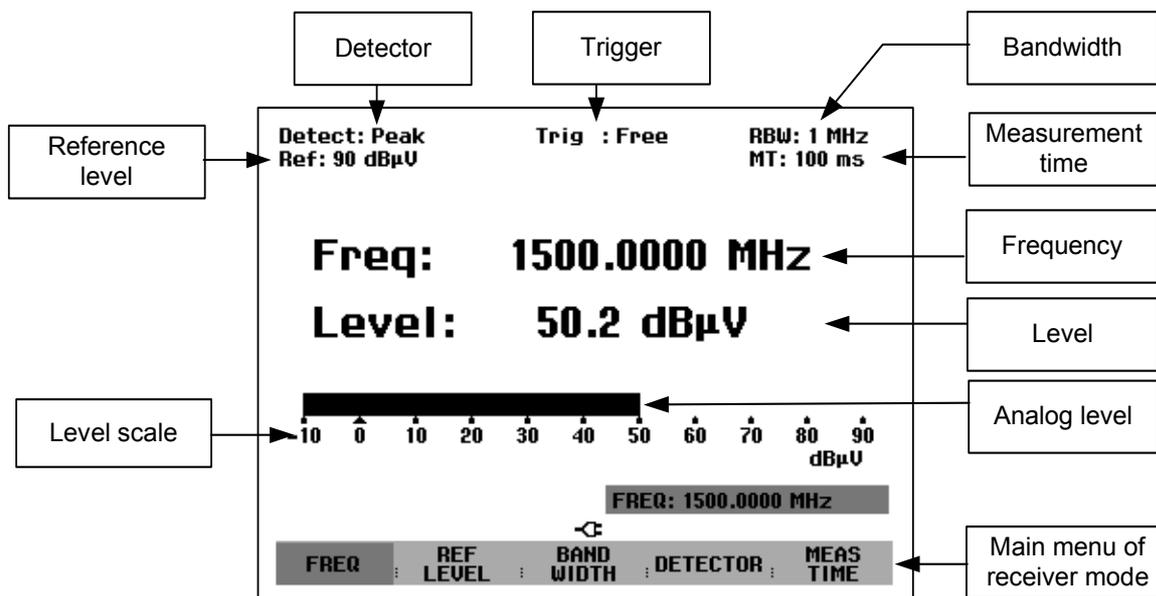
The R&S FSH provides the most important setting parameters such as frequency, reference level, measurement bandwidth, detector and measurement time in the main menu of the receiver mode. However, the settings can also be made using the corresponding keys.
