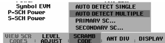
The scrambling code search takes about 50 s. The progress is indicated as a percent figure on the display. As soon as it has found the scrambling codes, the R&S FSH synchronizes to the 3GPP signal with the highest level. The screen will show SYNC OK, and the result values will be displayed.
