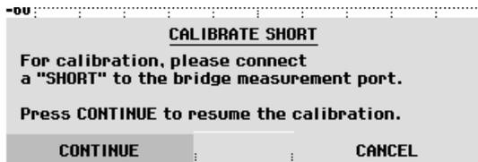
The third stage of the calibration process is connecting a 50 Ω termination to the measurement port.
