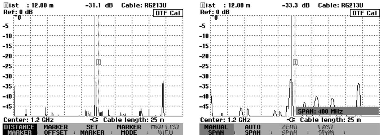
Measurement with automatic setting of the span (span = 2.025 GHz)      Measurement with 400 MHz span
