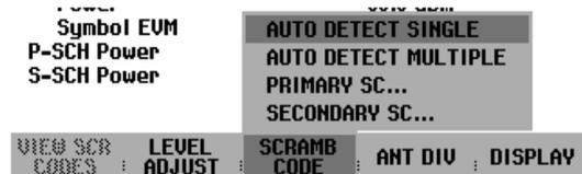
The scrambling code search takes about 22 s. The progress is indicated as a percent figure on the display. As soon as it has found a scrambling code, the R&S FSH synchronizes to the 3GPP signal of the base station. The screen will show SYNC OK, and the result values will be displayed.
