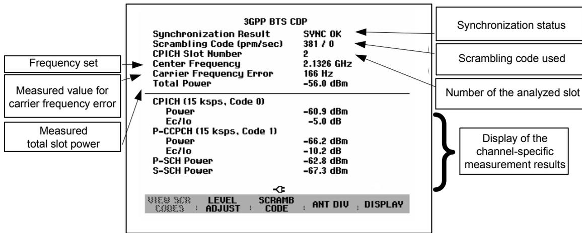
To simplify operation and to prevent incorrect measurements, the R&S FSH is equipped with an automatic routine for setting the reference level. After setting the carrier frequency to the 3GPP signal, you should first perform the level adjust.
