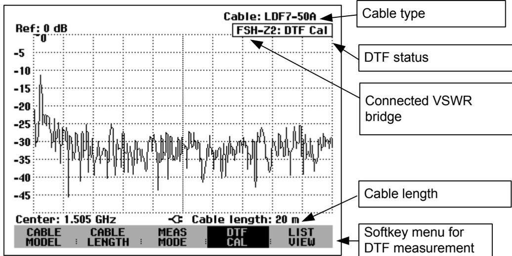
To perform distance-to-fault measurements, the R&S FSH needs to “know” the type of cable and its approximate length.
