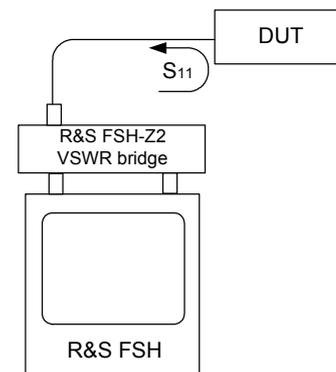
Fig. 2: Test setup for reflection measurements using the R&S FSH
