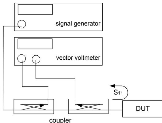
Fig. 1: Conventional test setup for reflection measurements using a vector voltmeter
