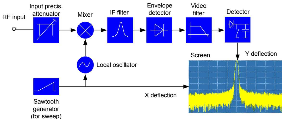
The precision attenuator at the input of the spectrum analyzer adjusts the level of the measurement signal to the level range that the mixer can handle without overdriving it. The precision attenuator at the input of the R&S FSH is adjustable in 10 dB steps from 0 dB to 30 dB and is directly coupled to the reference level setting.
