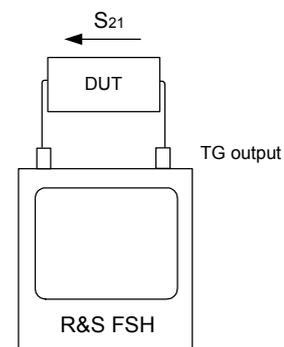
Fig. 4: Test setup for transmission measurements using the R&S FSH
