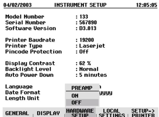
If the preamplifier is switched on, its use is coupled to the reference level, thus ensuring the optimum dynamic range of the R&S FSH at all times. The table below shows the positions of the RF attenuator and the preamplifier as a function of the reference level.
