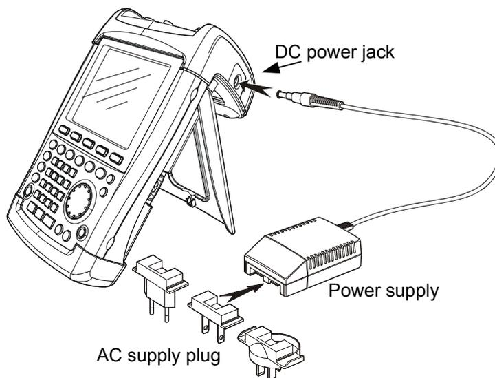
For rapid charging, be sure to switch off the R&S FSH during charging. The charging time is approx. seven hours. After four hours, the battery will be approx. 80 % charged.
