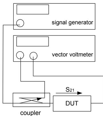
Fig. 3: Conventional test setup for transmission measurements using a vector voltmeter
