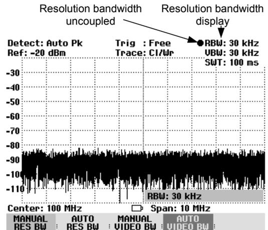
*Note: The 200 kHz resolution bandwidth has to be entered by means of the number keys. When using the rotary knob or the cursor keys, the 200 kHz bandwidth will be skipped.*
