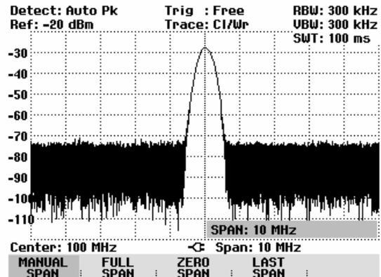
Use the FULL SPAN softkey to select the full span from 0 Hz to 3 GHz (R&S FSH3), from 0 Hz to 6 GHz (R&S FSH6) or from 0 Hz to 18 GHz (R&S FSH18) with a single keystroke.
