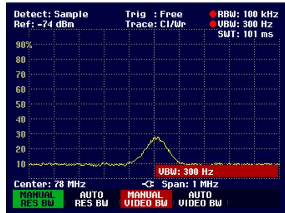
Limiting the video bandwidth smooths the trace considerably. This makes it much easier to determine the level of the measured signal.
