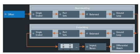
Figure 8-4: De-/Embedding calculation flow
