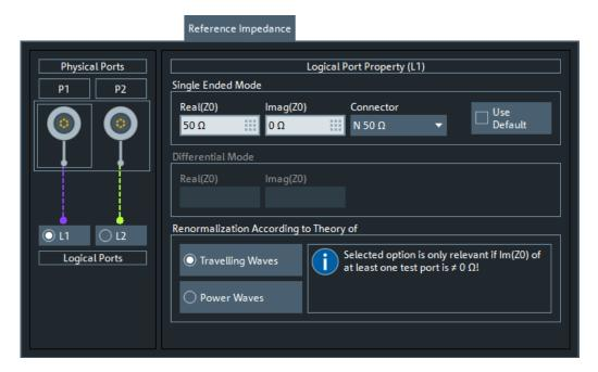
By default, the reference impedance of a physical port is set to the reference impedance of the connector type assigned to the port. However, it can be defined as an arbitrary complex value (renormalization of port impedances). By changing the reference impedance, it is possible to convert the measured values at 50  $\Omega$  (75  $\Omega$ ) into values at arbitrary port impedances.
