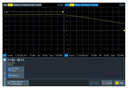
The analyzer performs a calibration sweep for the measured quantity  $S_{21}$ . The magnitude and phase of the result is displayed in two diagrams, together with the expected typical result for a Through standard. The similarity of real and expected traces indicates that the Through standard has been properly connected. After the R&S ZNL/ZNLE has completed the calibration sweep and calculated the correction data, the "Apply" button is enabled.
