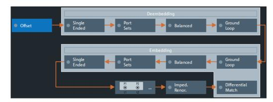
Figure 9-17: Offset Embed dock widget: Overview (Calculation Flow)
