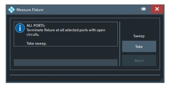
Figure 9-19: Measure Fixture dialog: Auto Length (and Loss)
