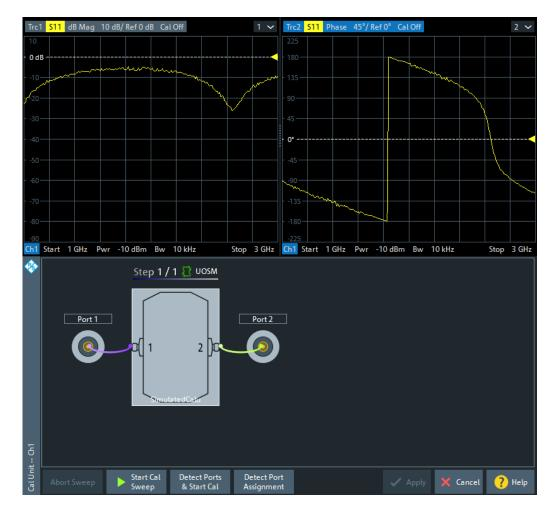
In the upper part of the "Cal Unit" screen, the R&S ZNL/ZNLE shows the calibration sweep diagrams for the currently measured S-parameter. The lower part visualizes the active port assignment and the measurement progress.
