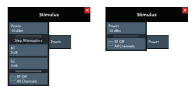
left = R&S ZNL with Receiver Step Attenuators right = R&S ZNLE (or R&S ZNL without Receiver Step Attenuators)
