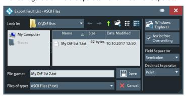
This CSV type file contains one line (terminated by CR+LF) per fault. With ";" as "Field Separator" and "." as "Decimal Separator", the fault list of Figure 9-4 is exported to
