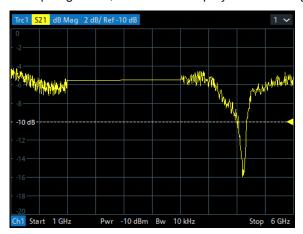
**Tip:** You can change to point based x-axis to improve the display of a segmented frequency sweep (see "Seg X-Axis" on page 309).
