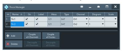
All existing traces of the current channel setup are listed in a table with several editable (white) or non-editable (gray) columns.
