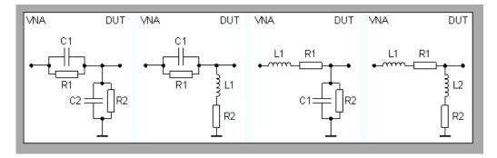
The following networks are composed of a shunt C or L (as seen from the analyzer port), followed by a serial C or L. They are named Shunt C, Serial C / Shunt C, Serial L / Shunt L, Serial C / Shunt L, Serial L.
