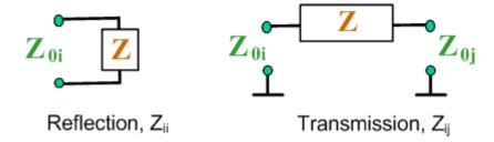
The analyzer converts a single measured S-parameter to determine the corresponding converted impedance. As a result, converted Z-parameters cannot completely describe general n-port DUTs:
