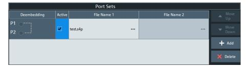
The "Port Sets" panel can also be activated by selecting the Port Sets Tab. Refer to its description for background information, parameters and additional remote commands.
