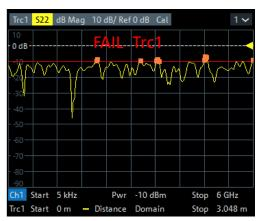
**Note** that the fault limit is handled like any other limit line. When "Fault Limit Check" is enabled, the current "Fault Limit" forms a new upper line segment replacing other previously defined limit lines (see Chapter 9.9.4.2, "Define Limit Lines Dialog", on page 402).
