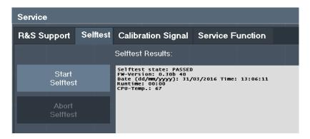
Once the self-test is started, all modules are checked consecutively and the test result is displayed. You can abort a running test.
