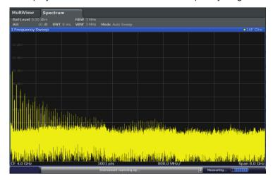
Figure 5-11: Calibration signal as RF input
