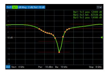
The limit line rules for logarithmic sweeps and segmented frequency sweeps with point-based x-axis also apply to ripple limit lines (see Chapter 8.4.1.1, "Rules for Limit Line Definition", on page 231).
