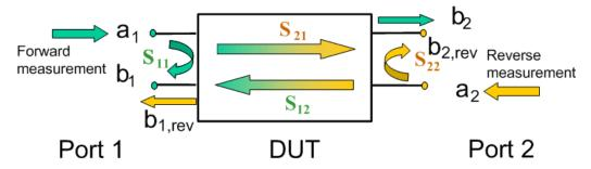
S<sub><mout><min>11</sub> is the mixed mode input reflection coefficient, defined as the ratio of the wave quantities b<sub>1</sub> (mode mout) to a<sub>1</sub> (mode min), measured at PORT 1 (forward measurement with matched output and a<sub>2</sub> = 0).
