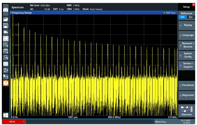
Figure 5-12: Calibration signal with optimized display settings
