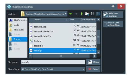
On loading data from a trace file with several traces, the analyzer displays a dialog to select one or more of the traces stored in the file (see Chapter 9.6.11.3, "Select Parameter Dialog", on page 361). E.g., for an \*.s2p Touchstone file, the box offers all four 2-port S-parameters (see Chapter 8.4.2.1, "Touchstone Files", on page 238).
