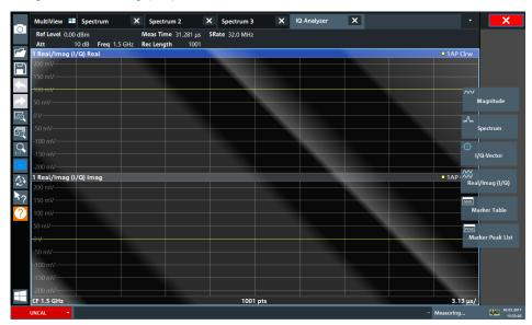
Figure 5-9: Inserting a Real/Imag diagram for I/Q analysis
