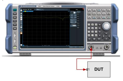
You can also use the basic transmission test setup, e.g. if you want to measure reflection and transmission parameters in parallel.
