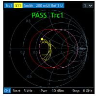
left ("FAIL") = "Circle Test" enabled, but not limited to "Display Circle" right ("PASS") = "Circle Test" enabled, but limited to "Display Circle"
