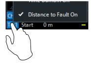
E.g. "Distance to Fault" can also be enabled/disabled via the context menu of the trace label (touch and hold for more than one second).
