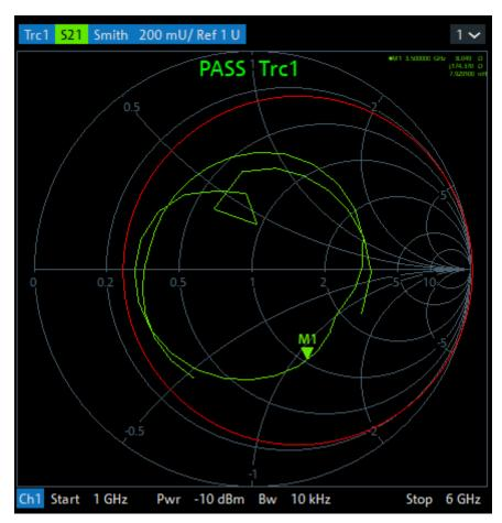
With a circle limit line centered on the left border of an inverted Smith diagram (Y = infinity), you can check whether the imaginary part of the admittance (Im(Y), susceptance) falls below a limit.
