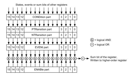
The sum bit is obtained from the EVENt and ENABle part for each register. The result is then entered into a bit of the CONDition part of the higher-order register.
