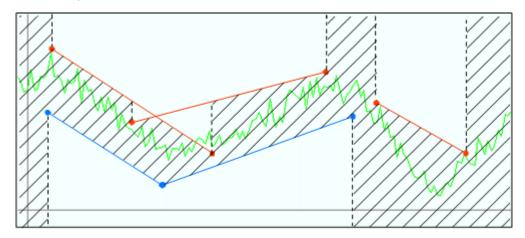
As a consequence of the limit line rules, a DUT always passes the limit check if no limit lines are defined.
