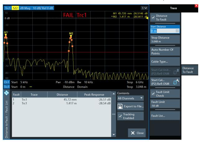
The frequency sweep may have to be adjusted to the length of the transmission line and the expected distance to fault:
