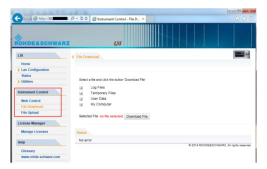
The most commonly used folders on the instrument are displayed, for example those that contain user data, as well as the top-most  ${\tt My}$  Computer folder, from which you can access all other folders on the instrument.
