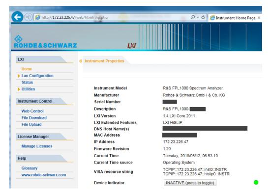
The instrument home page displays the device information required by the LXI standard including the VISA resource string in read-only format.
