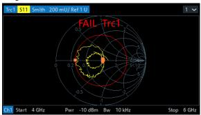
Figure 9-10: Simultaneous dB Mag limit line and circle check
