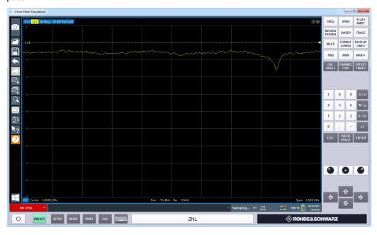
To activate or deactivate the front panel temporarily, press the [F6] key on the external keyboard (if available) or the remote computer.
