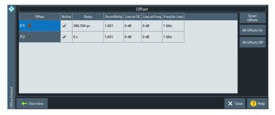
Figure 9-18: Offset Embed dock widget: Offset panel
