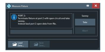
Figure 9-20: Measure Fixture dialog: Direct Compensation (and Prompt for Each Port)
