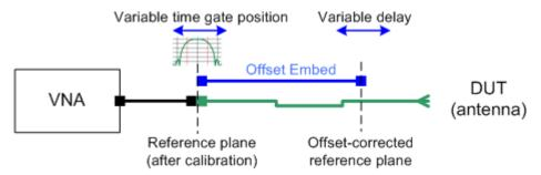
If "Adjust Time Gate" is on, the time gate is moved to left (right) when the offset-corrected reference plane is moved to the right (left). Its absolute position remains fixed. With this setting, it is possible, e.g., to keep the time gate at the position of the antenna connector while the antenna is measured at different length offsets.
