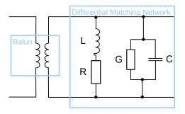
In contrast to standard balanced embedding (4-port), the matching circuit is only applied to the differential mode port (2-port). It can be specified via a Touchstone s2p file or by parametrizing a lumped "Shunt L, Shunt C" element model.
