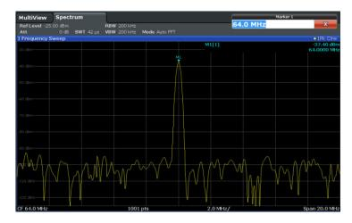
6. Now you can move the marker by tapping and dragging it to a different position. The current position is indicated by a dotted blue line. Notice how the position and value change in the marker area of the diagram.
