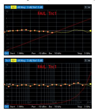
While "Show Limit Line" is active, the diagrams display all limit line segments.
