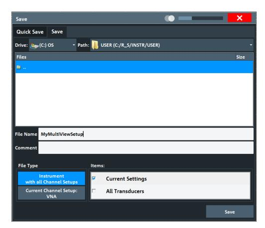
Figure 5-7: Saving the instrument settings to a file
