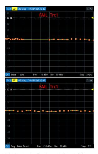
**Tip:** Overlapping limit line and ripple limit line segments are not displayed when a point-based x-axis is active; see Chapter 8.4.1.1, "Rules for Limit Line Definition", on page 231.
