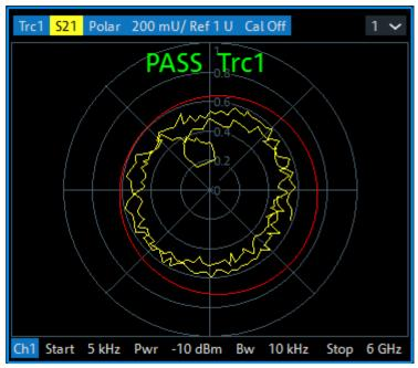
With a circle limit line adjusted to the right border of a Smith diagram (Z = infinity), you can check whether the imaginary part of the impedance (Im(Z), reactance) falls below a limit.
