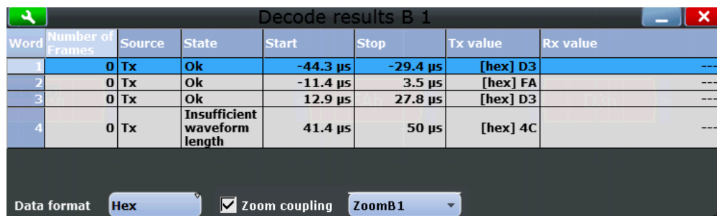
Figure 12-11: Decode results of the UART signal
