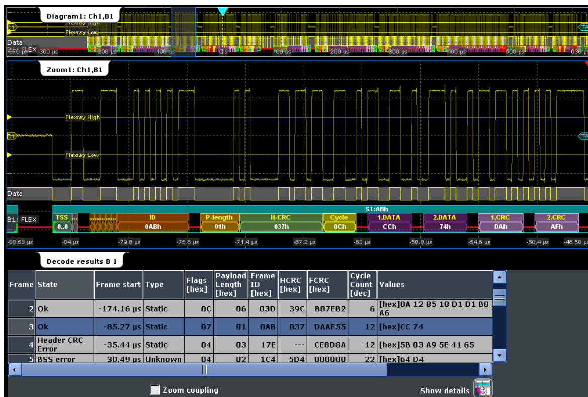
Figure 12-37: FlexRay - decoded dynamic slot and results table
