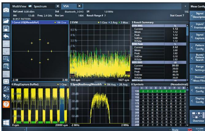
Demodulation of a DVB-SX2 multi-modulation signal with the R&S®FPL1-K70M option (R&S®FPL1-K70 option required)
