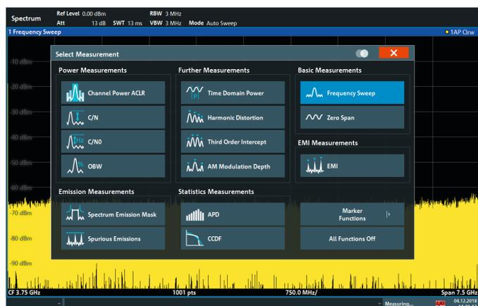
The R&S®FPL1-K9 option and an R&S®NRP power sensor turn the R&S®FPL1000 into a power meter
